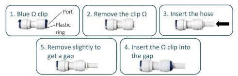
**To disconnect:** Remove the clip  $\Omega$ , push the plastic ring against the fitting to release the hose. Remove the hose from the fitting.
